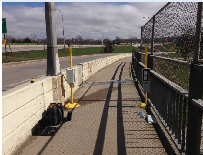
Figure 13: Microwave Detector Installation using Stanchions
