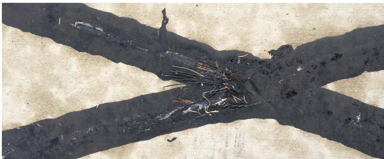
Figure 18: Inductive Loop on Top of Road Surface Worn and Frayed from Exposure and Road Maintenance
